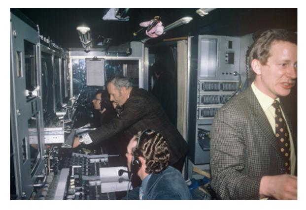
In 1969 the BBC was in the process of moving from black and white to colour technology and commissioned a number of new colour scanners. These were called CMCR (Colour Mobile Control Room) vehicles.
