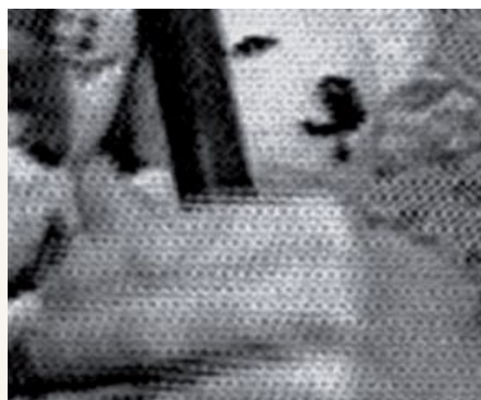
Original colour video recording and 'chroma dots' in a non-filtered B&W telerecording
